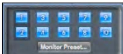
The monitor control enable buttons indicate which outputs are controlled by the monitor section on the GUI directly below the ten buttons. The Saffire PRO 40 can be set up so that you have hands-on control of volume levels, and depending on your monitoring set-up, you may control no speakers, just a single pair of speakers, or up to 10 speakers simultaneously.
