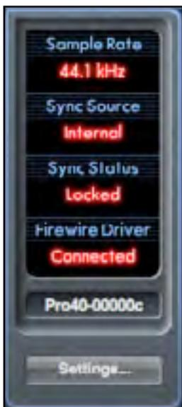
The Device Status section shows information about the sample rate, synchronisation and driver status of the Saffire PRO 40. The desired sample rate can be set as well as external synchronisation options for using the Saffire PRO 40 with external digital devices.
