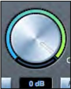
Set the output level of all assigned outputs using this knob. The output level can be adjusted using the mouse, or from the front panel control, depending on the status of the H/W Control button. The dB display below shows the current level to which the monitor knob is set.
