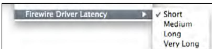
The Saffire PRO 40s latency performance will be dictated by the Core Audio buffer size specified in your DAW (Mac,) or as set in the ASIO buffer size (Windows.) The Firewire Driver Latency affects the performance of the Core Audio or ASIO buffer settings.
