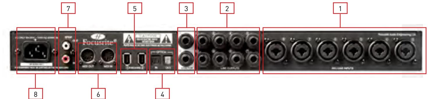
1. 6 Combo XLR input sockets for Mic / Line. – Each socket will accept an XLR, or 1/4 inch TRS (balanced) or TS (unbalanced) Jack connector.
