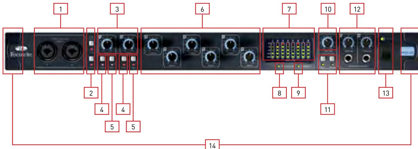
1. Channel 1 and 2 Combo XLR input sockets. Each socket will accept an XLR, or 1/4 inch TRS (balanced) or TS (unbalanced) Jack connector
