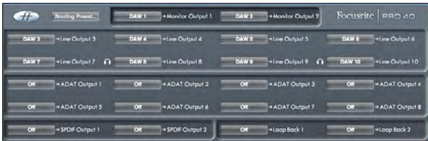
The routing section allows you to set up which audio sources are to be routed directly to which physical outputs.
