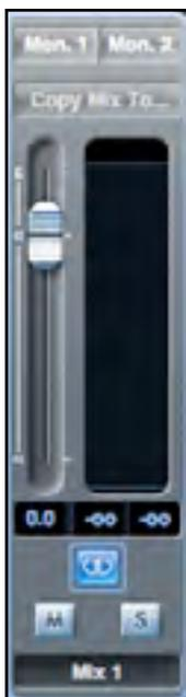
The output channel of the mixer is where all the input channels are routed to and mixed together. The output channel gives you control of the overall level of the entire mix.
