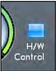
When lit, the monitor knob on the front panel takes control of the monitor level control knob. Mouse control of the monitor knob is disabled when active.
